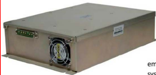
Kuerzi Avionics' powerful AC-DC converter with three-phase, 115-volt input and variable frequency, with an output of 28 volts and 1,000 watts
